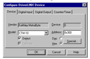
Use the Device subsystem page to tell DriverLINX the model name, address and, optionally, to disable detection and testing of your CTM Series board.
