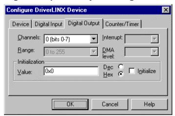
Use the Digital Output subsystem page to change the default digital output channel initialization values.
