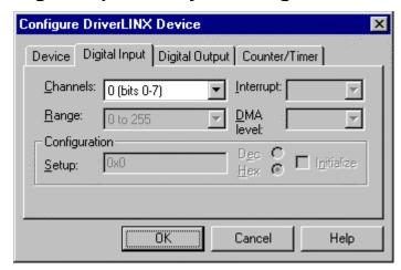
For the Keithley CTM Series, there are no configuration settings on the Digital Input Subsystem page. You can view the list of Logical Channels and their ranges.
