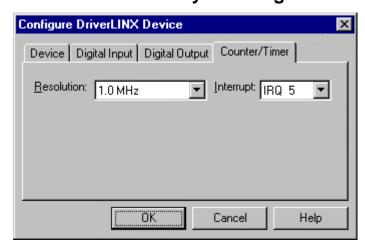
Use the Counter/Timer subsystem page to select the internal master clock frequency that the hardware inputs to the prescaler for the counter/timer channels and to define the interrupt channel, if any, for the counter/timers. Enter selections for the following fields:
