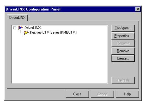
When you click the *Create... or Configure...* buttons on the *DriverLINX Configuration Panel*, DriverLINX displays the *Configure DriverLINX Device* dialog. The dialog has a page for each subsystem on a Keithley CTM Series model. The following sections describe your choices in configuring DriverLINX to work with your board.
